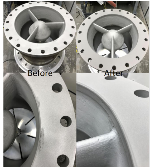
This fielded light water reactor component was repaired with cold spray as part of a collaborative effort with VRC Metal Systems and Exelon.
