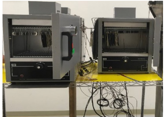
Special ovens are used to accelerate the aging of components, such as electrical cables, that are exposed to extreme environments inside nuclear power reactors.
