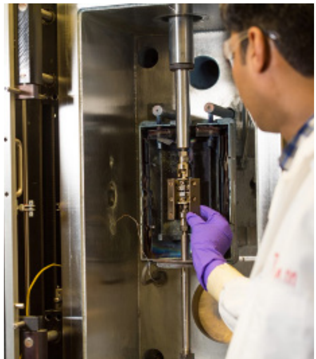
PNNL materials scientists evaluate the mechanical properties of nuclear materials using an Instron tensile tester with an atmosphere-controlled high-temperature Centorr furnace.
