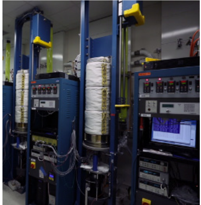
PNNL's Stress Corrosion Cracking (SCC) Laboratory contains multiple SCC initiation test measurement systems designed and built by PNNL researchers to identify the onset of SCC in pressurized water nuclear reactors.
