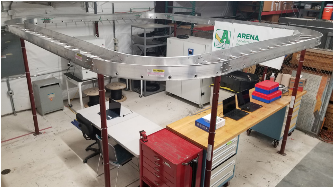
Researchers use the ARENA Cable/Motor Test to evaluate the integrity of the wide variety of cables used inside extreme environments, including nuclear power plants.
