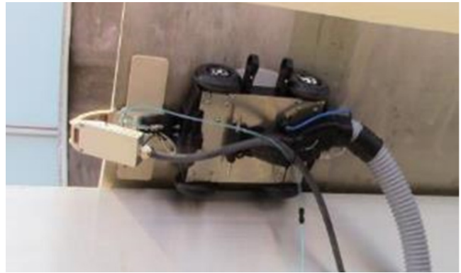
Development of a remote inspection system for spent nuclear fuel storage casks is in progress at PNNL, which will help identify the aging mechanisms associated with chloride-induced stress corrosion cracking.
