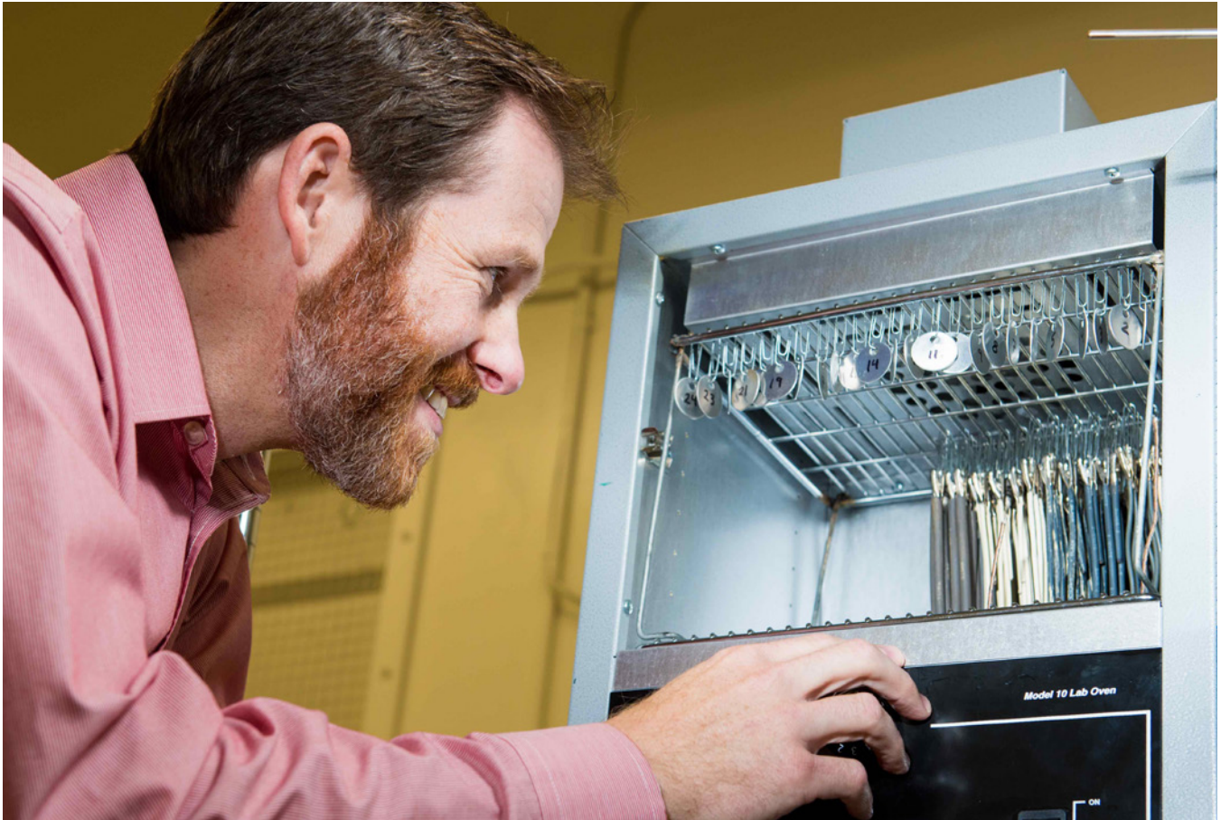
Cable samples undergo temperature and high gamma testing in PNNL's High Exposure Facility, as part of a reactor life extension research project for the DOE Office of Nuclear Energy.
