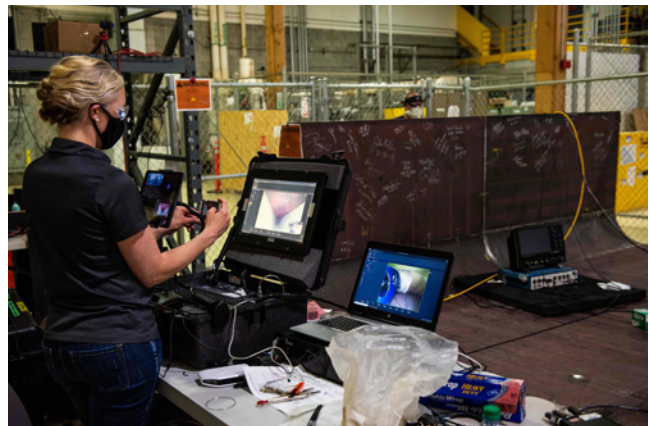
In partnership with industry and DOE contractors, PNNL is demonstrating an Electro Magnetic Acoustic Transducer (EMAT) system for inspecting aging underground double-walled radioactive waste storage tanks.
