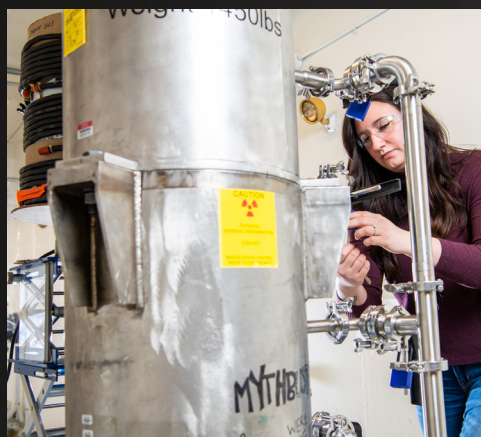
Long-term high-dose irradiation for cable aging studies
