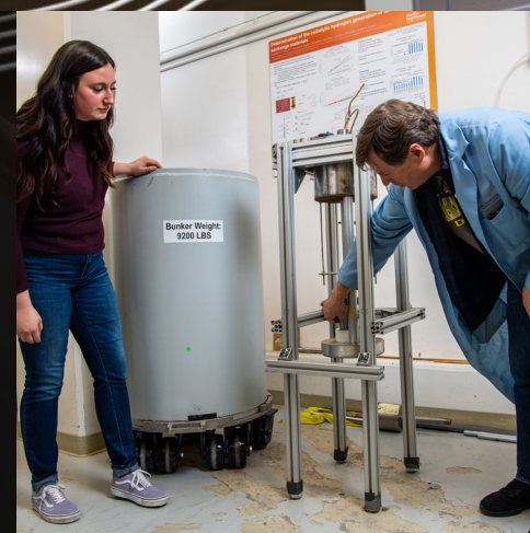
Lead Shielded Gamma Bunker
