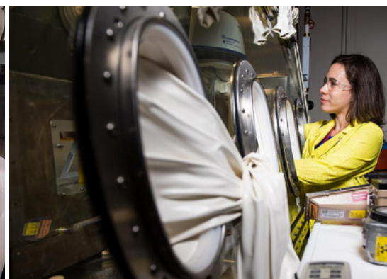
Researchers use glove boxes, hot cells, radiological fume hoods, and specialized equipment in RPL
