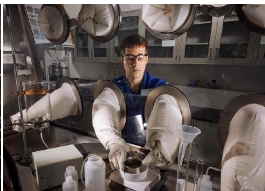
Researchers use glove boxes, hot cells, radiological fume hoods, and specialized equipment in RPL
