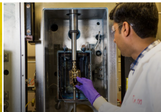
Evaluating the mechanical properties of nuclear materials using an Instron tensile tester
