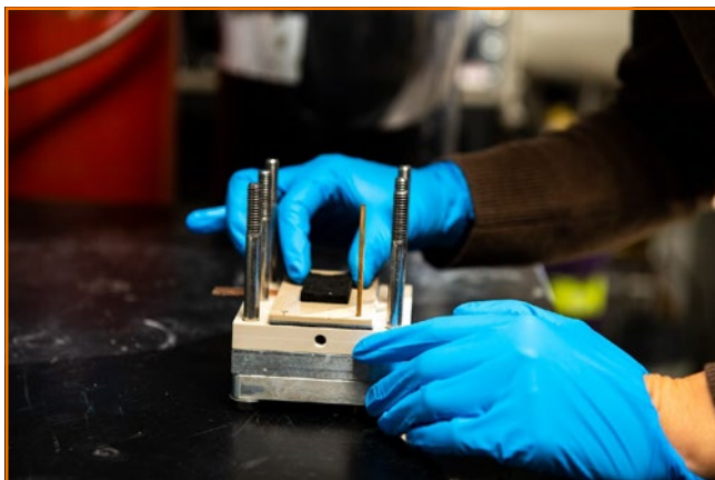
A thin titanium foil catalyst coated with ruthenium oxide nanoparticles in the anode helps convert the biocrude to useful oils while also transforming compounds to more atmosphere-friendly gasses. Photo: Andrea Starr
