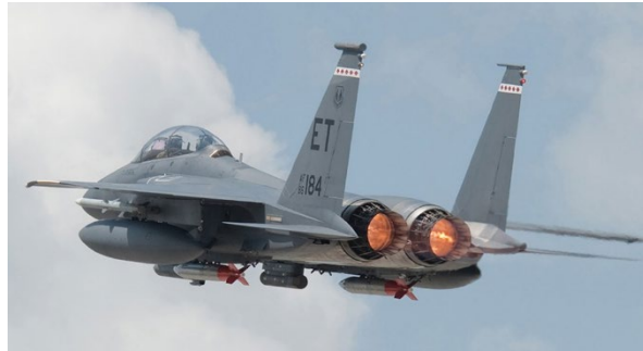
An F-15E conducts a vibration fly-around test for the B61-12 Life Extension Program.
