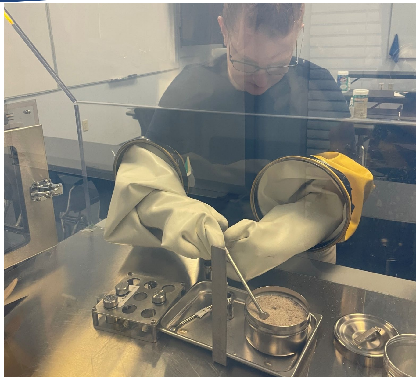
Paige demonstrating safe material handling in a glovebox used for SRS's Plutonium Training Courses, one of many to be implemented in the High-Fidelity Training and Operations Center
